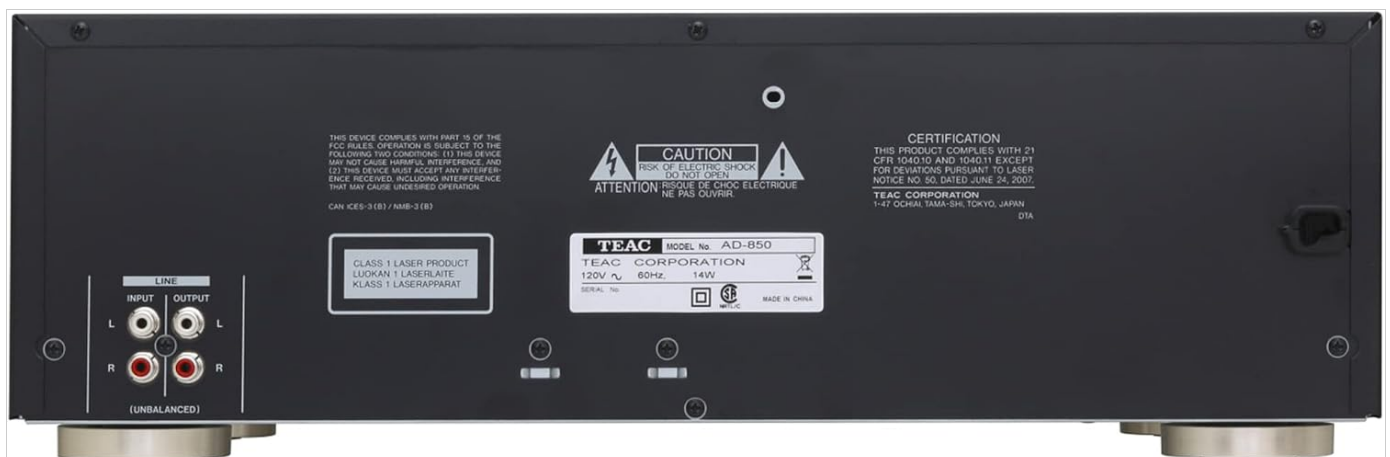
Figure 4.2: Rear view of the TEAC AD-850 unit, displaying the LINE INPUT and LINE OUTPUT RCA jacks, and the power input.
