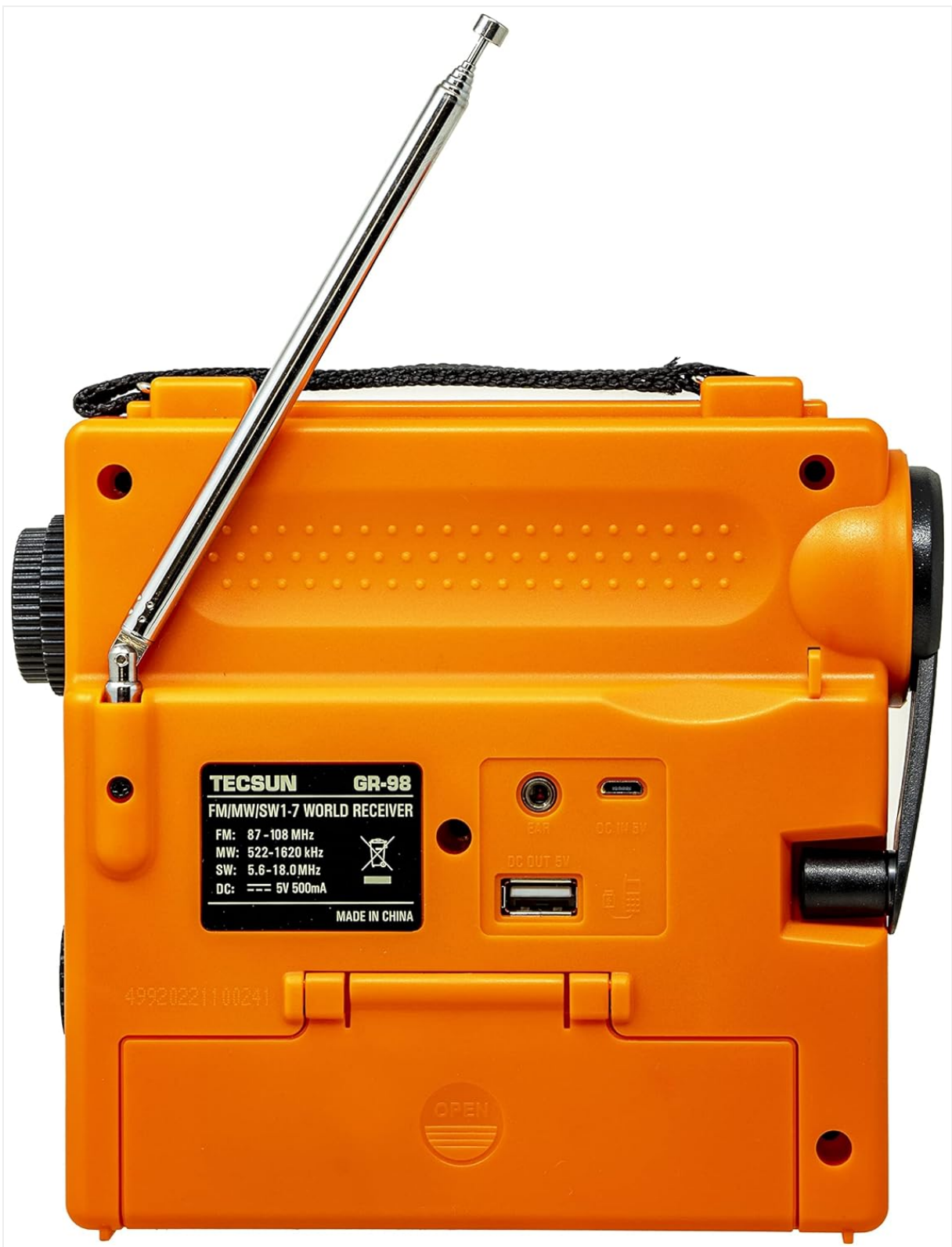
Figure 4.2: Rear view of the Tecsun GR-98, highlighting the connectivity ports: DC IN 5V (mini-USB), DC OUT 5V (USB-A), and the 3.5mm earphone jack.
