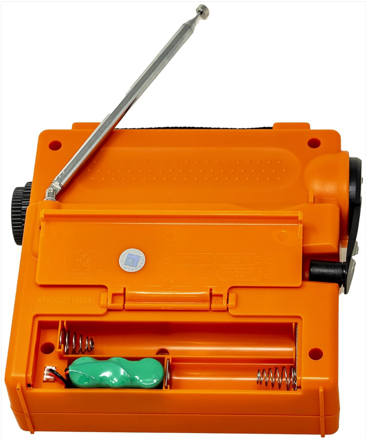
Figure 5.1: The battery compartment with the NiMH battery pack installed and slots for optional AA batteries.
