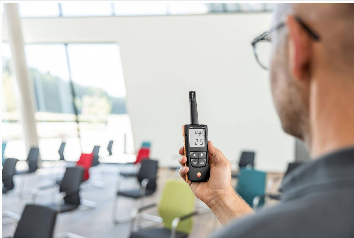
Figure 3: The Testo 625 Digital Hygrometer being used by a person in an indoor environment, demonstrating its portability.
