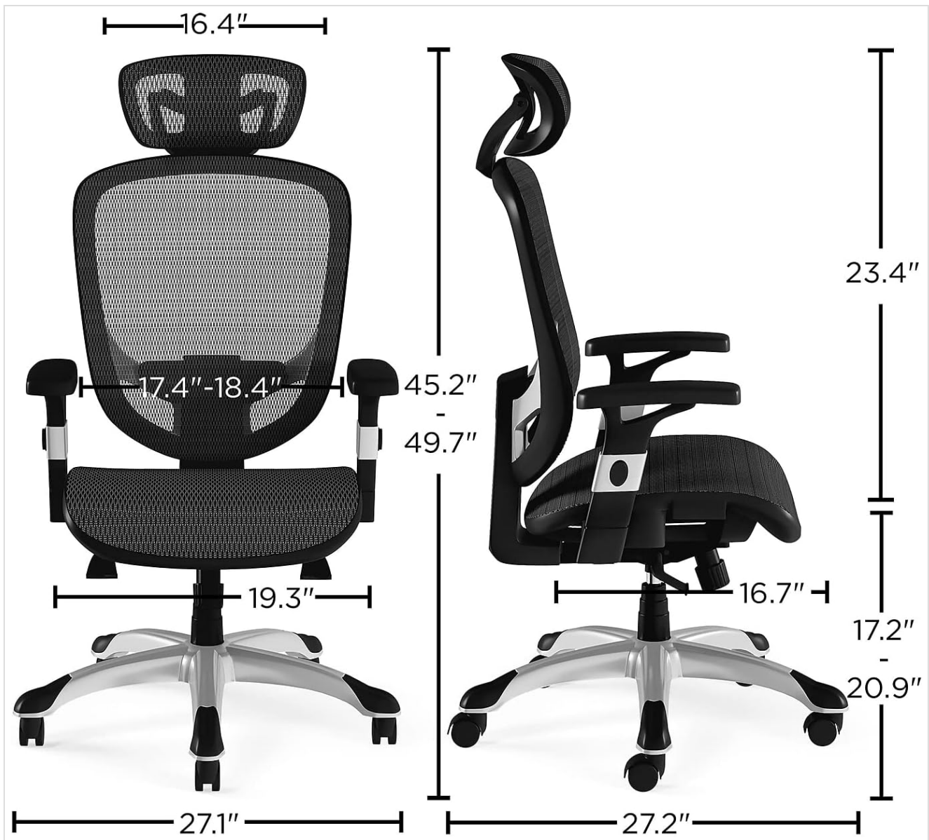
Figure 6: A diagram illustrating the overall dimensions of the chair, including height, width, depth, and seat height ranges.
