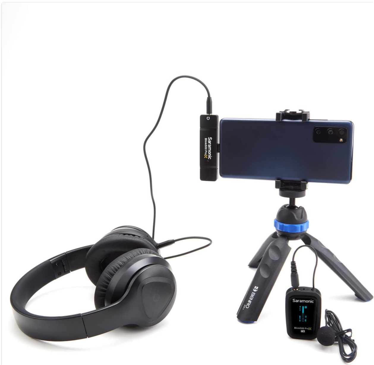
Image 4.1: Monitoring audio with headphones connected to the RXUC receiver.
