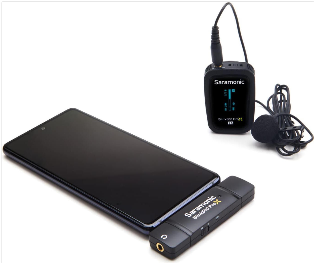
Image 3.2: The RXUC receiver connected to a mobile phone.
