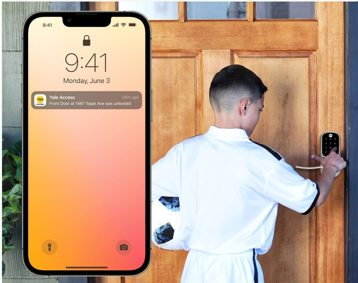
Figure 4: Remote access and status monitoring via the Yale Access App.
