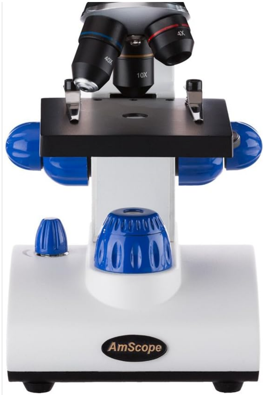
Image: Side view of the AmScope Student Microscope, illustrating the coarse and fine focus knobs.
