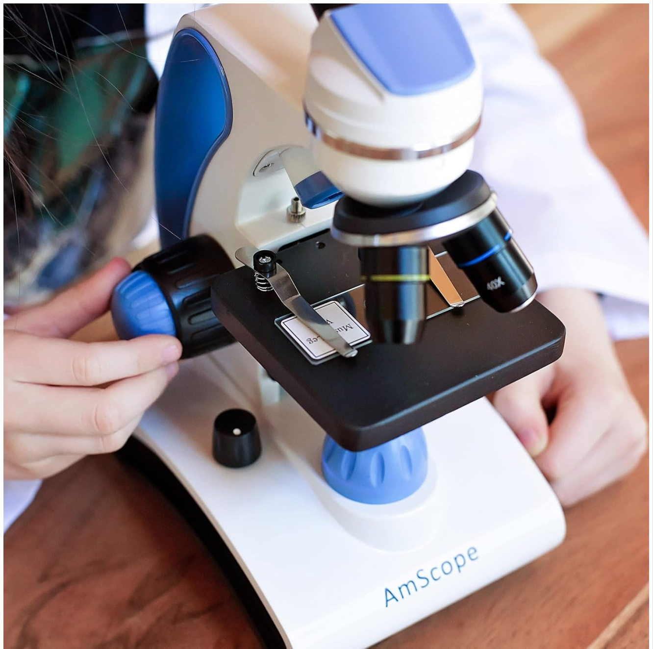
Figure 3: Demonstrating the use of focus knobs for clear specimen viewing.
