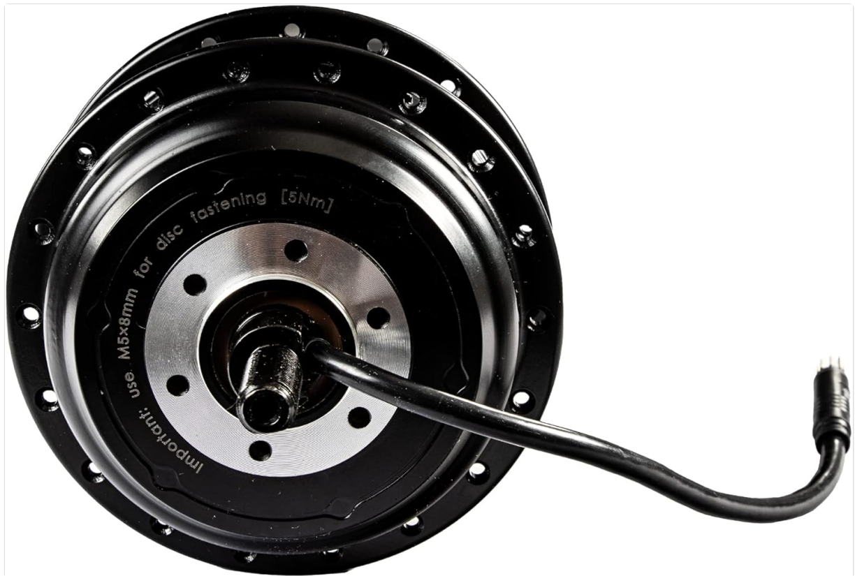
Figure 4.1: Motor cable exit and disc brake mounting. This view highlights the specific side for cable routing (left side) and the 6-hole pattern for attaching a disc brake rotor. Note the "important: use M5x8mm for disc fastening [5Nm]" text on the motor body.
