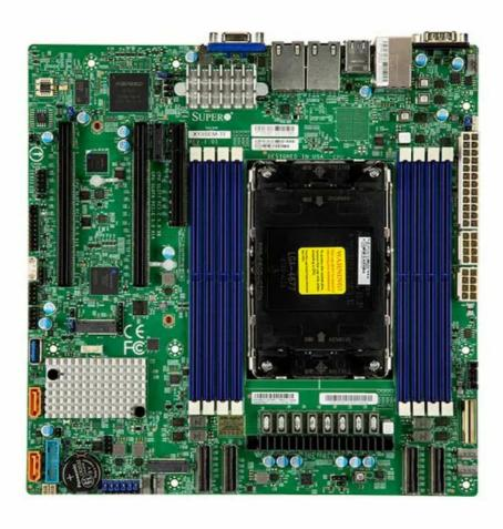
Image Description: This image displays the Supermicro X13SEM-TF motherboard. Key visible components include the large LGA 4677 CPU socket at the center, surrounded by eight DDR5 DIMM slots (blue). Various PCIe slots, SATA ports, USB headers, and power connectors are distributed across the green PCB. The rear I/O panel features USB ports, Ethernet ports, and a VGA port. Heatsinks are visible over the VRM and chipset
