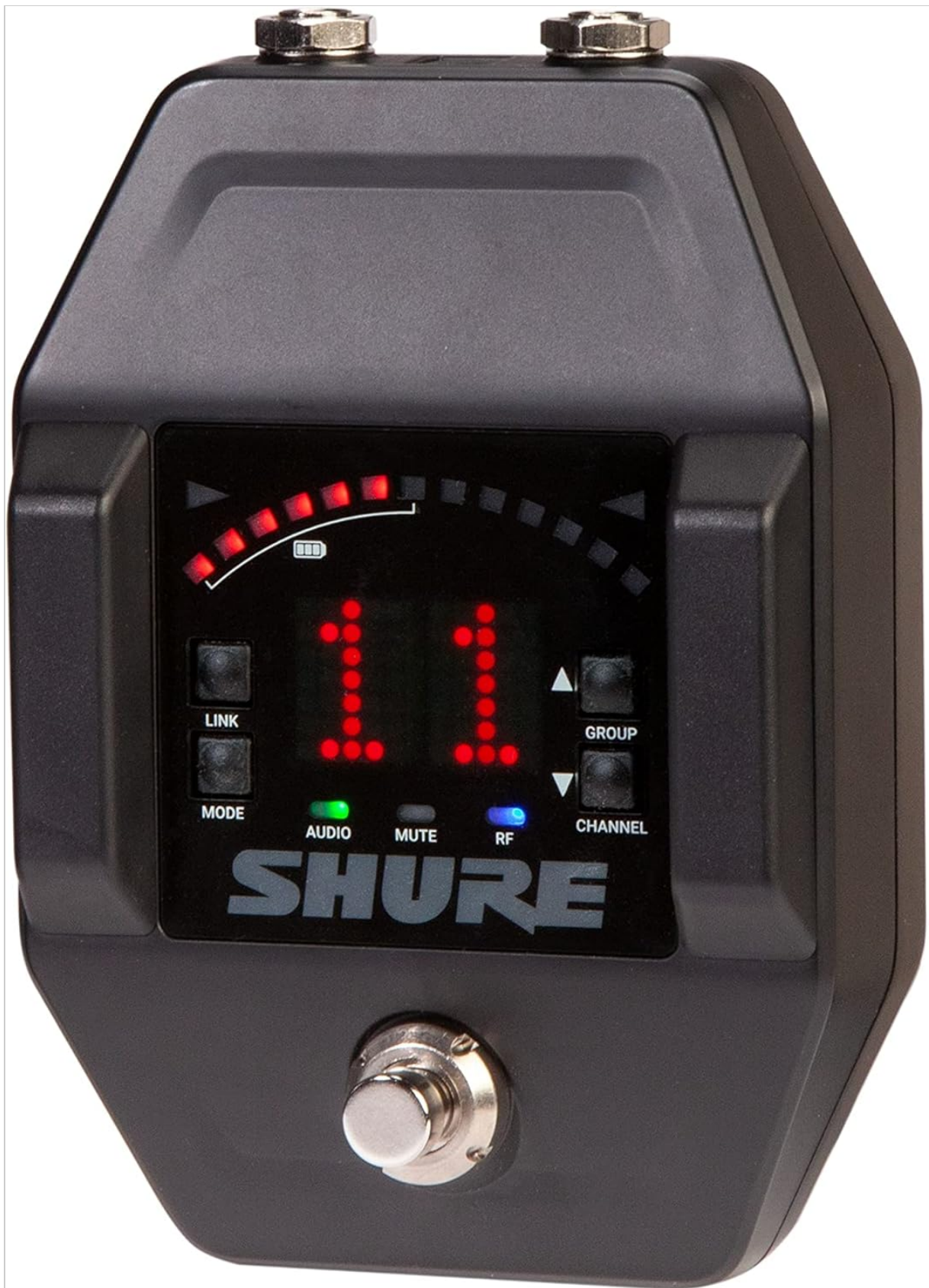
Front view of the GLXD6+ pedal receiver, highlighting the LED display for channel, group, and battery status, along with the mode, audio, mute, RF, and channel buttons.
