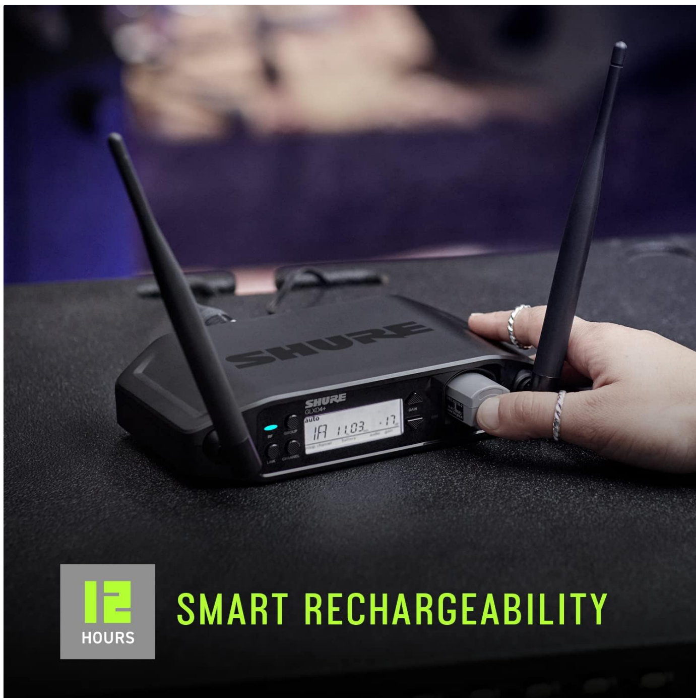
Figure 5: Charging the GLXD+ system via USB-C.
