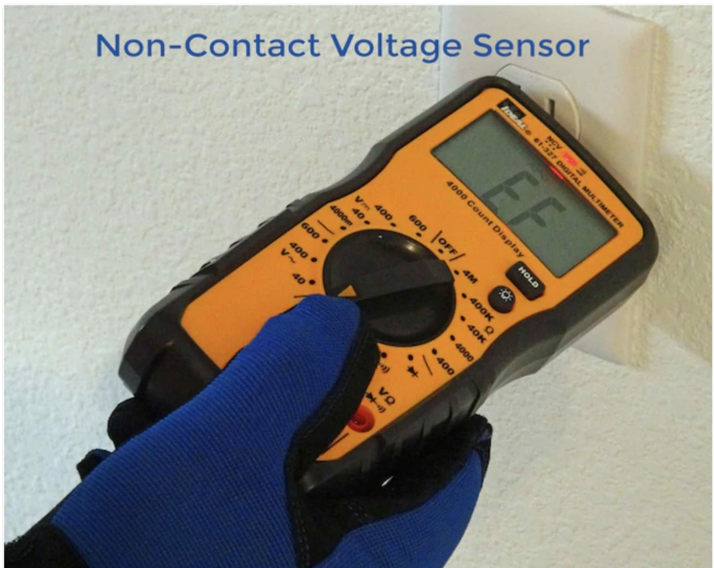
Figure 6.1: The multimeter being used to perform a Non-Contact Voltage (NCV) test near an electrical outlet. The display shows "EF" indicating voltage detection.
