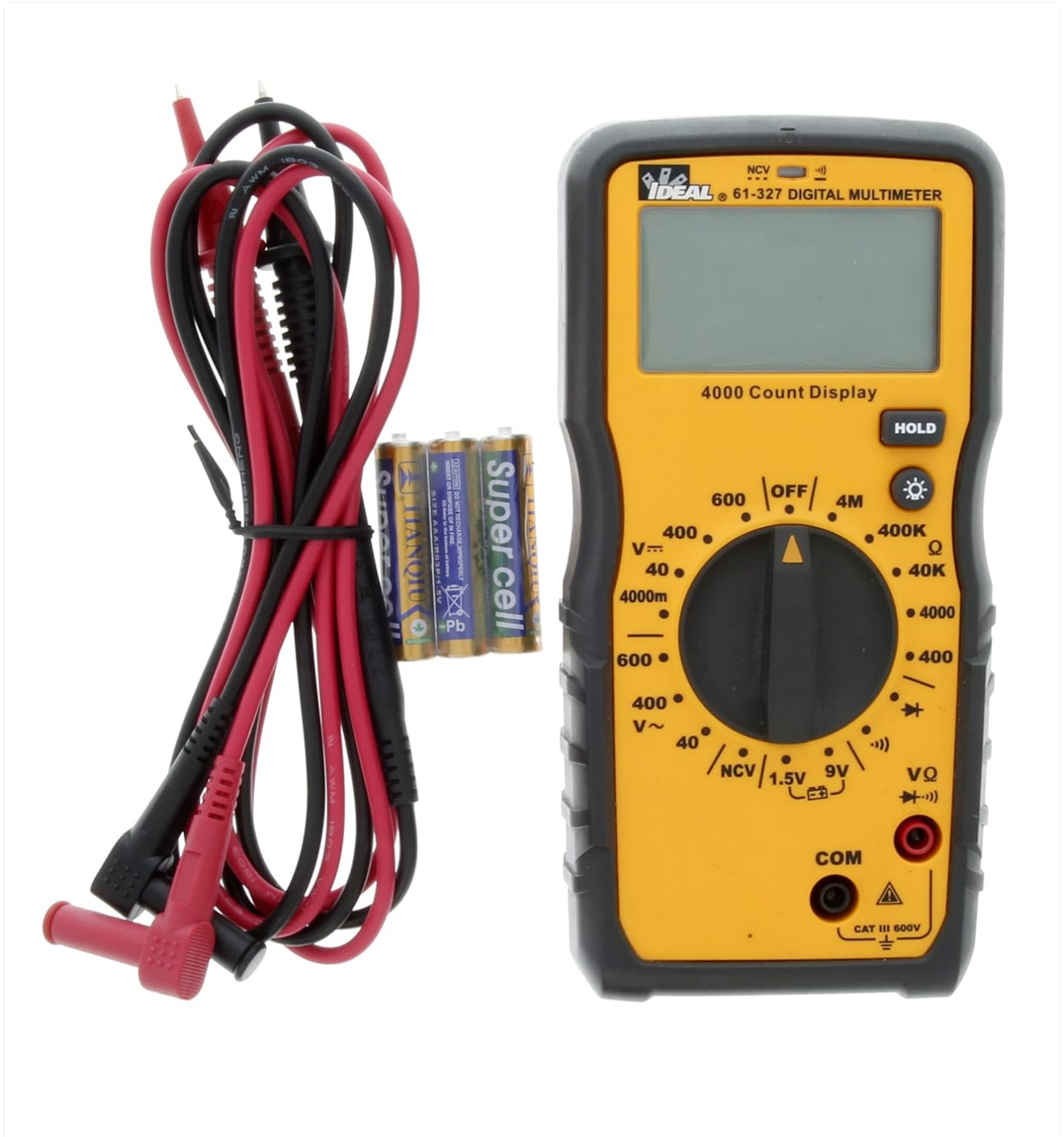
Figure 5.1: The multimeter shown with its test leads and batteries, ready for initial setup. The black lead connects to COM, and the red lead connects to VΩ.
