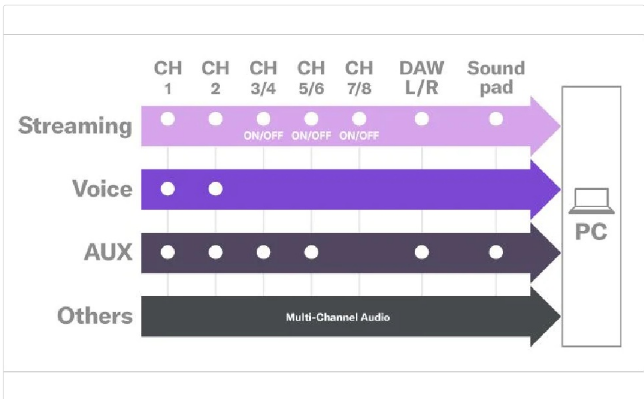
Figure 6: USB audio routing diagram, showing how different channels can be assigned for streaming, voice, AUX, and multi-channel audio to a PC.
