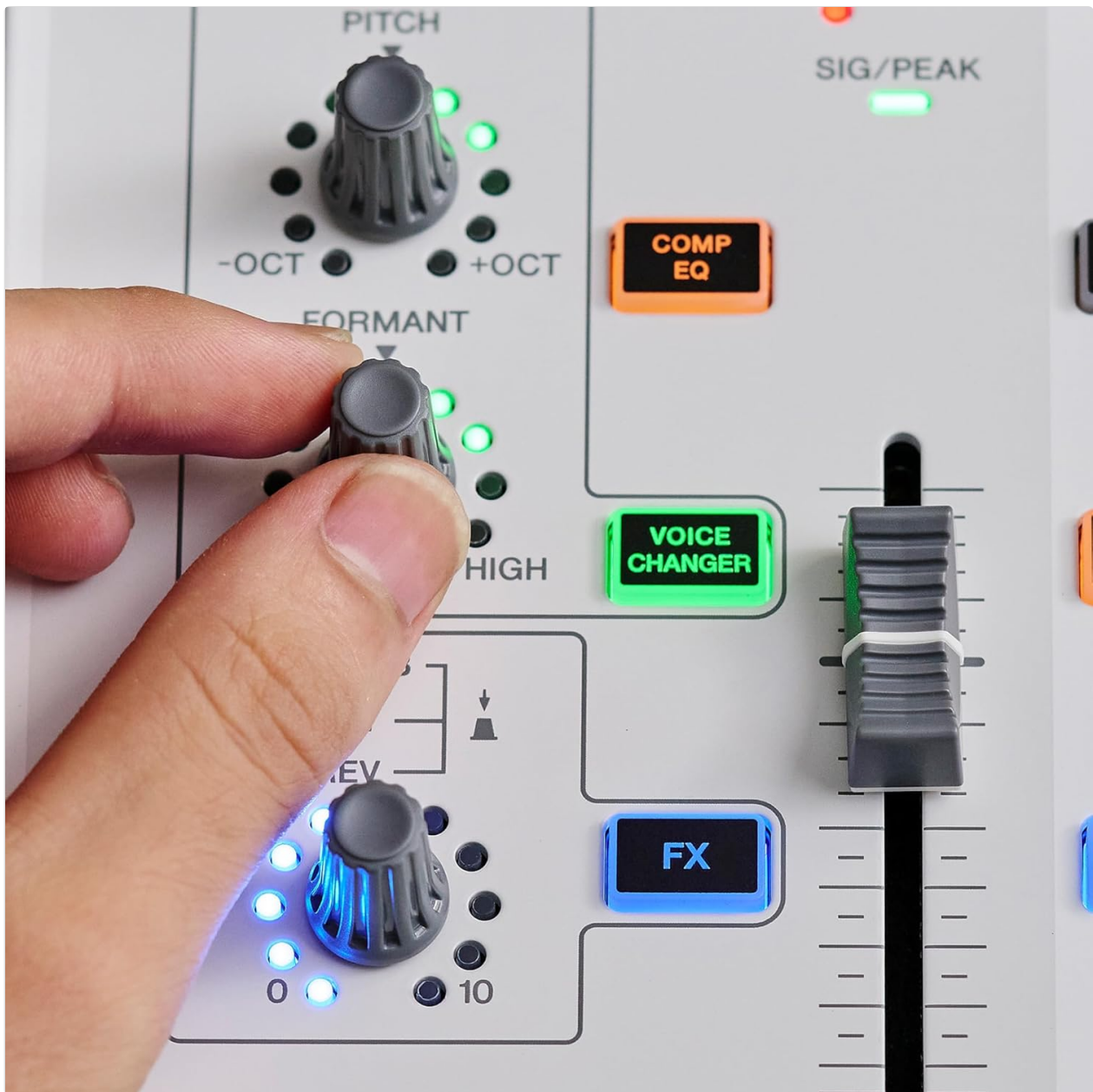
Figure 4: A hand adjusting a pitch/formant knob, highlighting the voice changer and effect controls.
