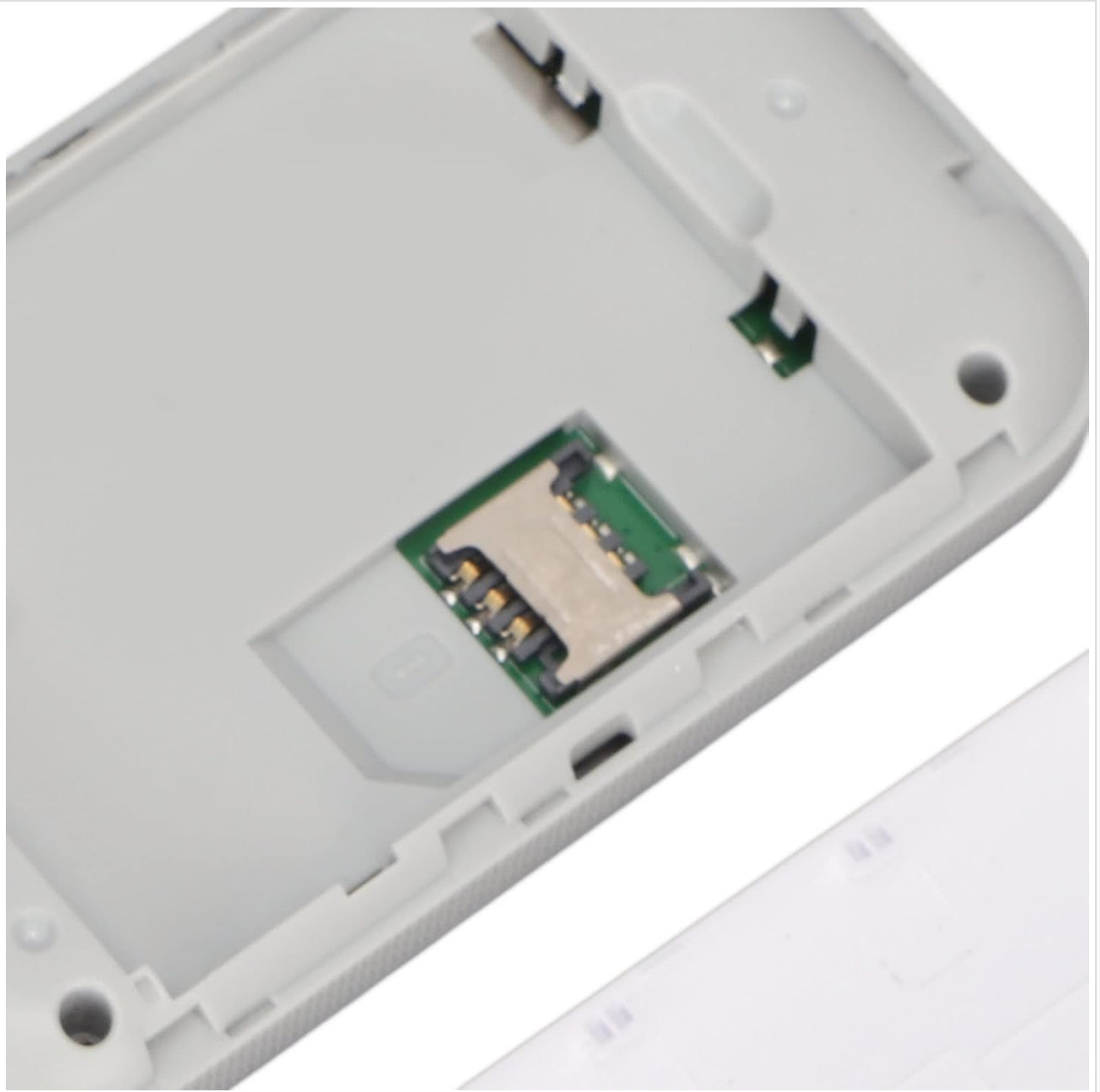
Figure 4: SIM Card Slot Detail. A close-up view of the router's internal SIM card slot, ready for a standard SIM card insertion.
