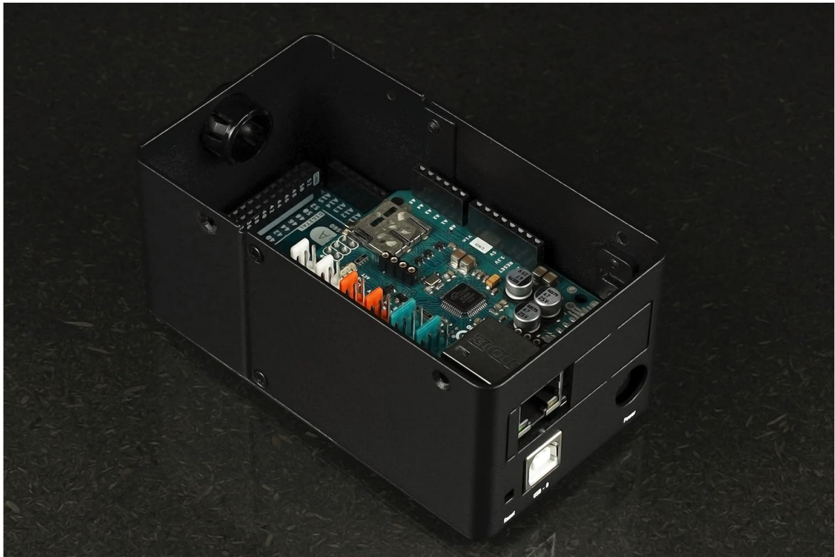
Figure 3: An Arduino board correctly installed within the KKS case, demonstrating proper alignment with internal mounting points and external port cutouts.
