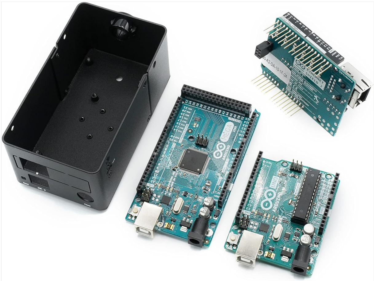
Figure 5: Components including the KKS case, an Arduino UNO, an Arduino Mega, and an Ethernet Shield, demonstrating compatibility and potential configurations.
