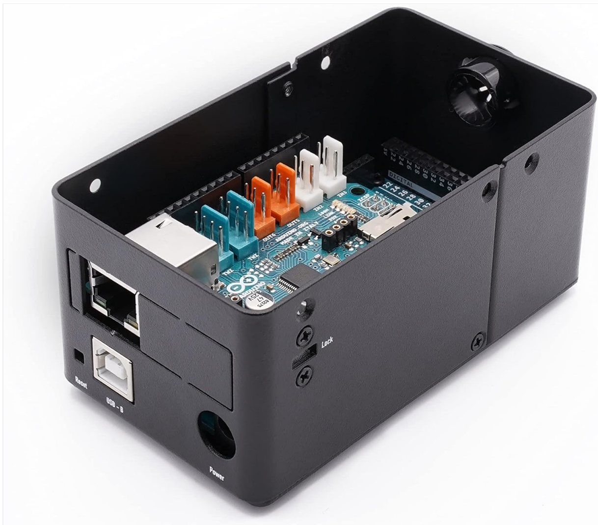
Figure 4: An Arduino board with an attached shield inside the KKS case, illustrating the ample space provided for additional components.
