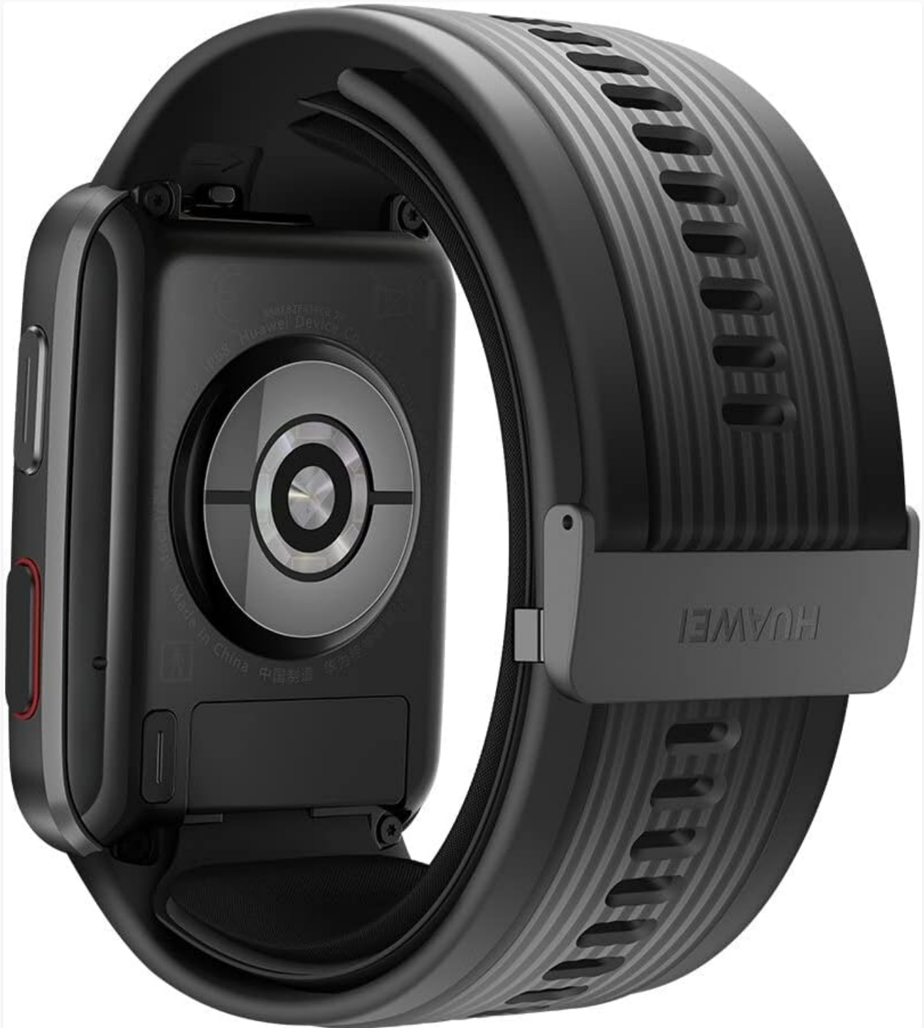
Image 2.1: The rear view of the HUAWEI Watch D, highlighting its sensors and the flexible strap.
