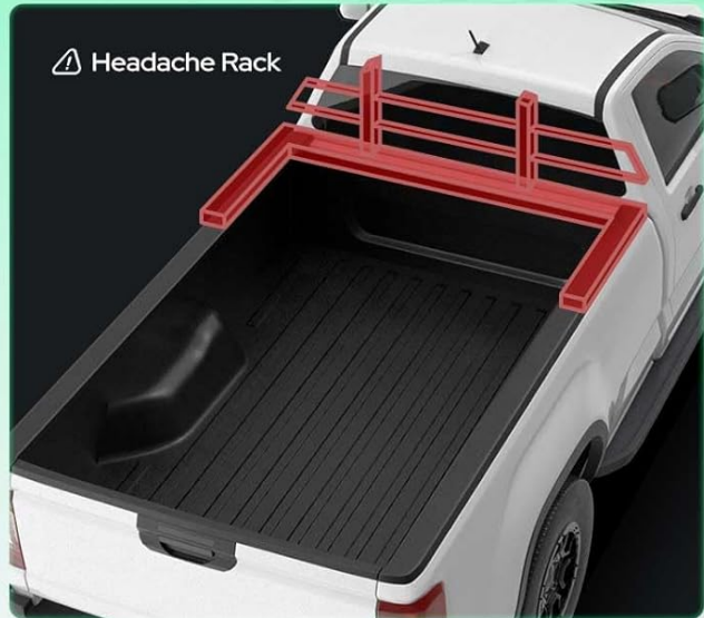
Figure 2.2: Examples of truck bed modifications that require removal.
