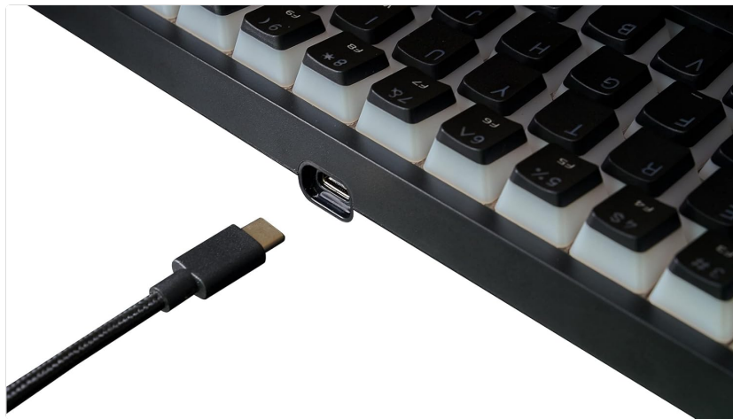
Figure 3.1: Connecting the USB Type-C Cable
