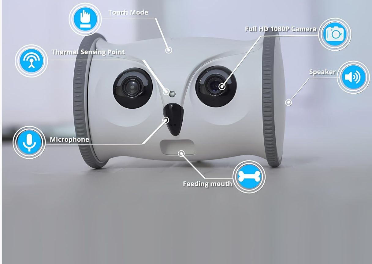
Figure 1: Product Exterior. This image displays the front view of the Owl Robot, highlighting key features such as the Full HD 1080P Camera, Microphone, Speaker, Thermal Sensing Point, Touch Mode indicator, and Feeding Mouth. The wheels are visible on either side.
