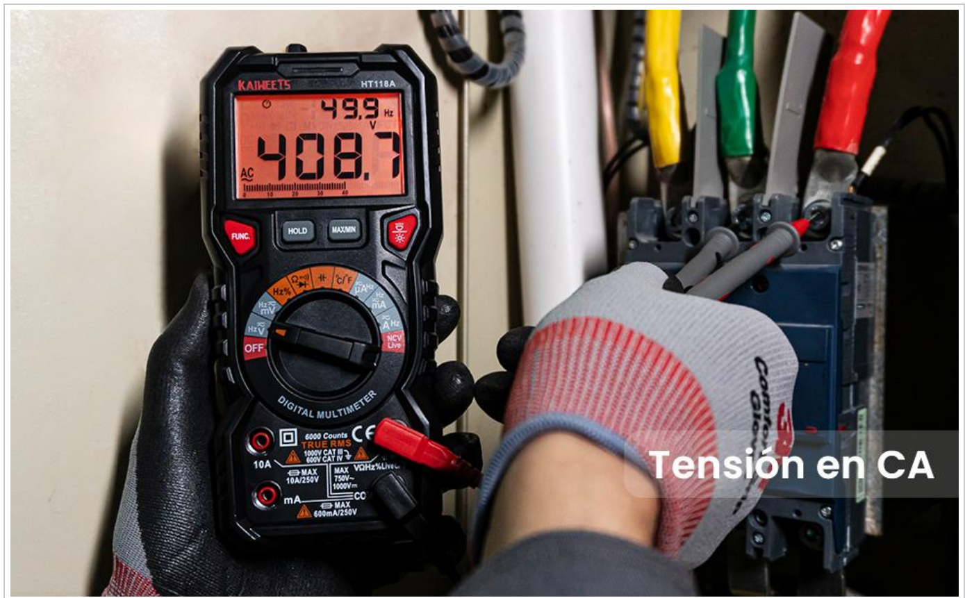
Figure 3: Measuring AC voltage with the HT118A multimeter.
