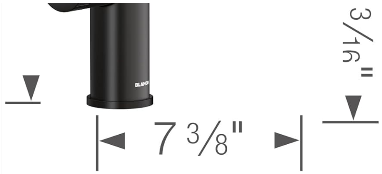
Figure 1: Faucet Dimensions. This image displays the key measurements of the faucet, including its overall height, spout height, and spout reach, which are approximately 19 1/8 inches, 6 3/16 inches, and 7 3/8 inches respectively.
