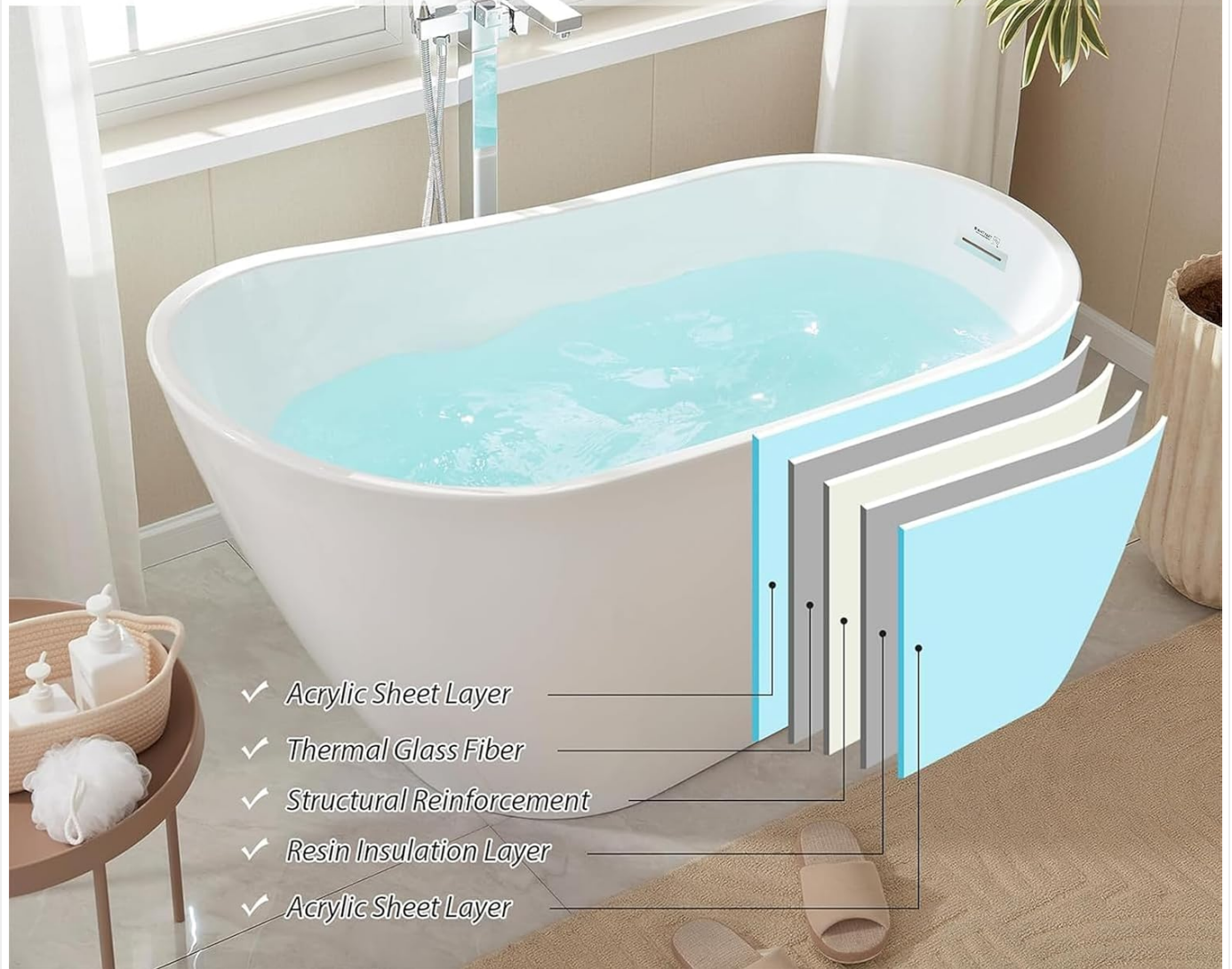
Figure 1.2: High Heat Retention Layers
