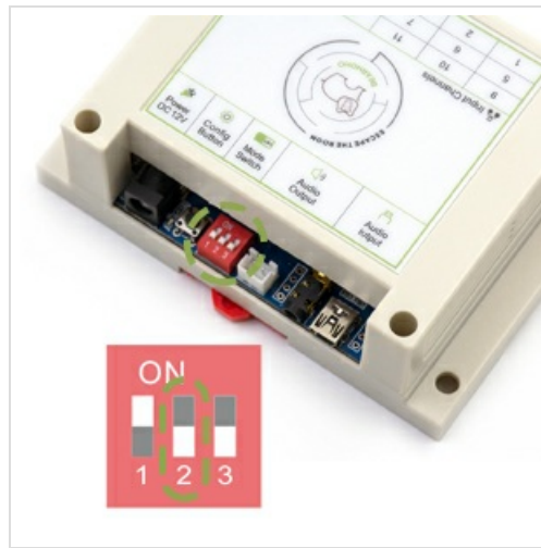
Figure 6: Location of the beep sound disable switch.
