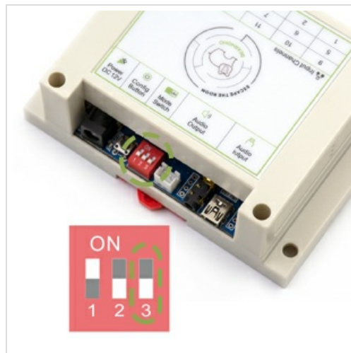
Figure 5: Controller DIP switches for reset mode configuration.
