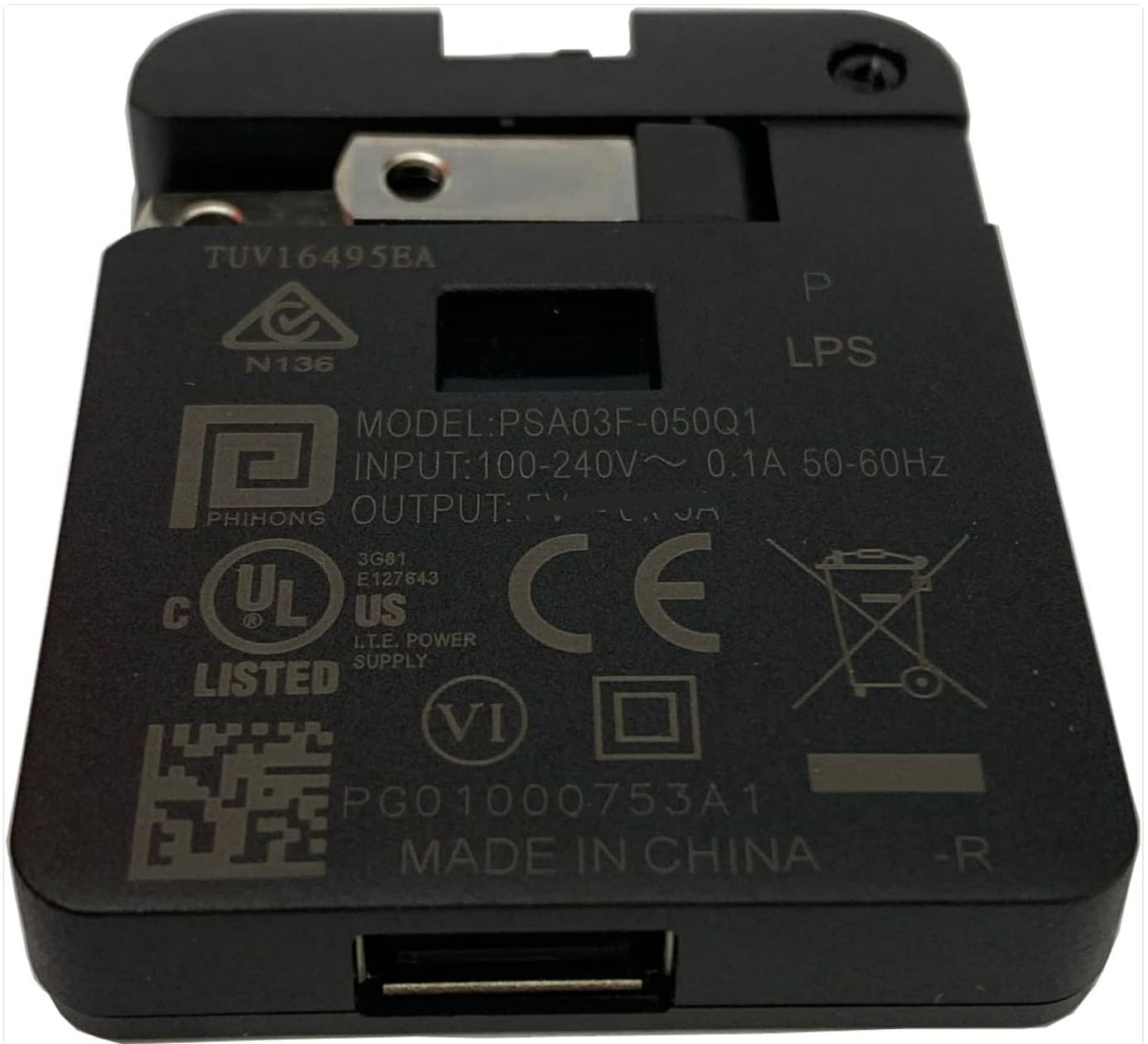
Image: A close-up view of the UpBright AC/DC adapter, showing its input and output specifications. The label indicates "MODEL: PSA03F-050Q1 INPUT: 100-240V~ 0.1A 50-60Hz OUTPUT: 5V."
