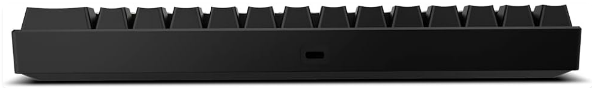
Rear view of the KROM KYARA keyboard, showing the central USB-C port for wired connection and charging.
