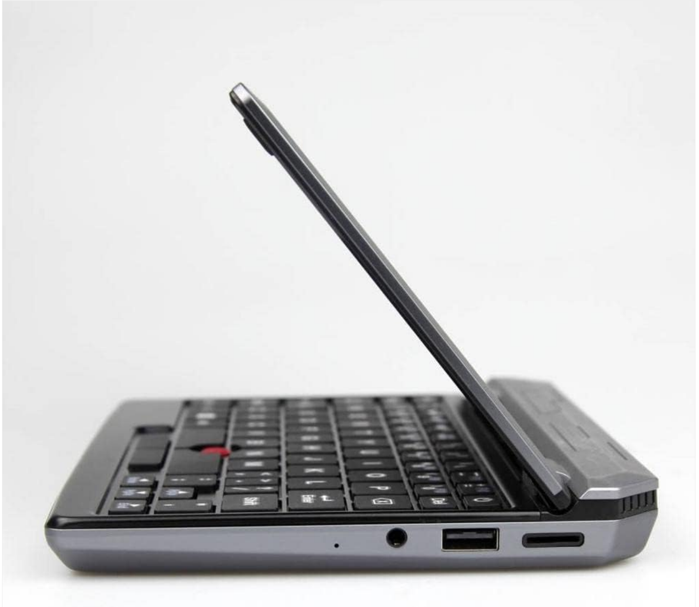
Image: Side view of the PiPO W7 Mini-Laptop, highlighting the audio jack, USB 3.0 port, and microSD card slot for easy access during setup.
