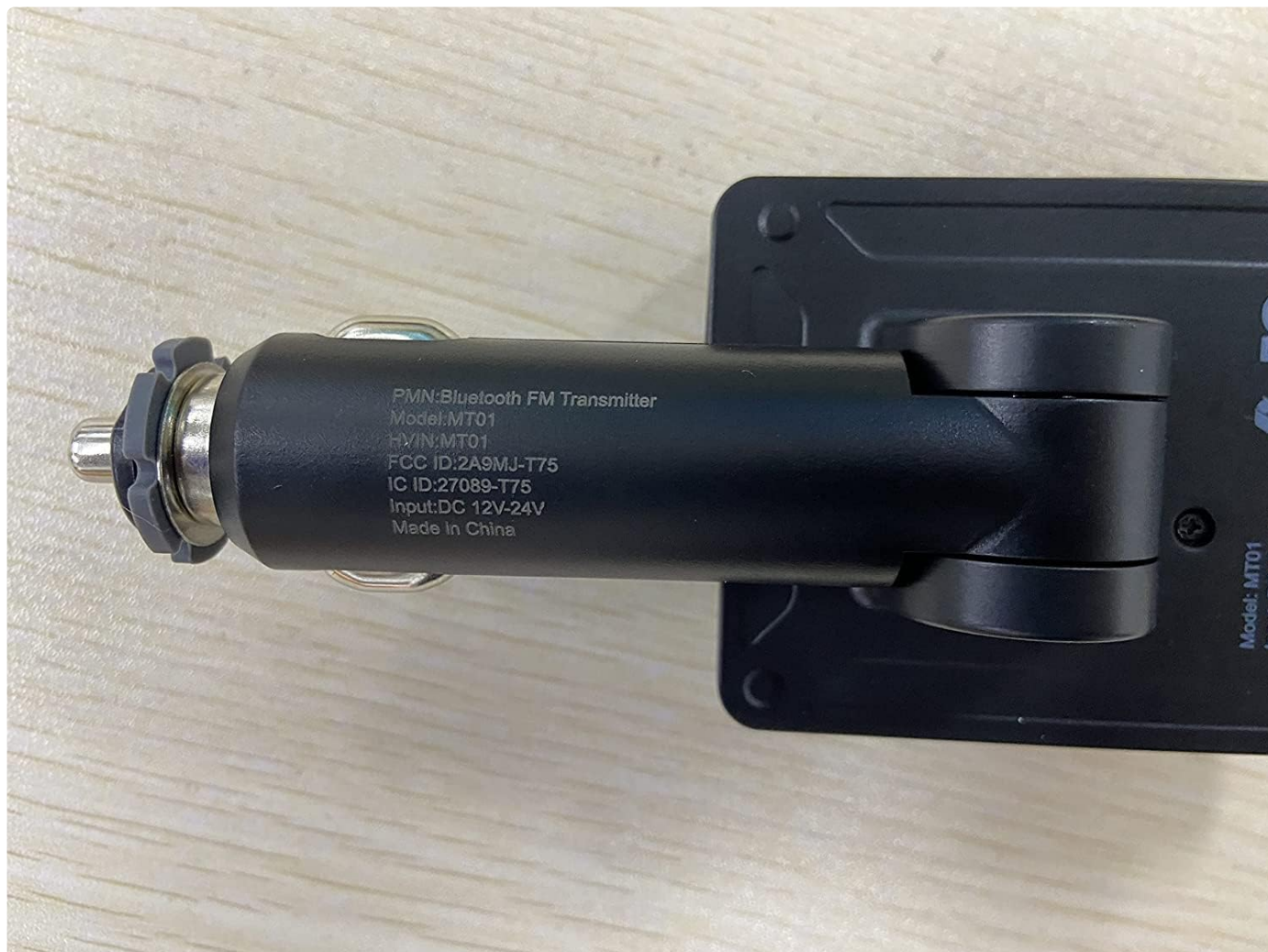
Image: The underside of the LENCENT FM Bluetooth 5.3 Transmitter, displaying its model number (MT01) and electrical input specifications.
