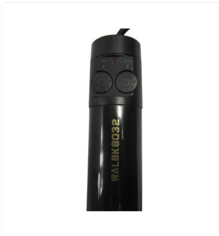
Figure 3: Control buttons for air volume and heater temperature on the hot air gun.
