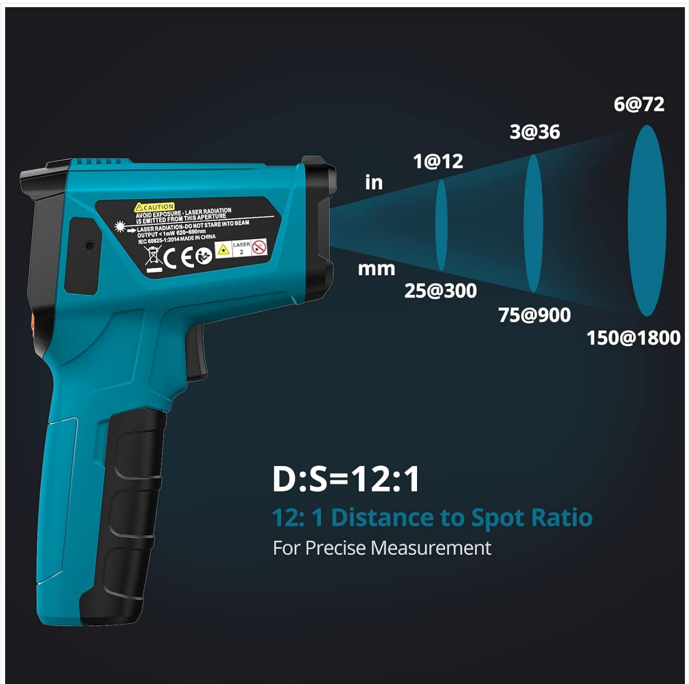
Figure 4: Understanding the 12:1 Distance to Spot Ratio.
