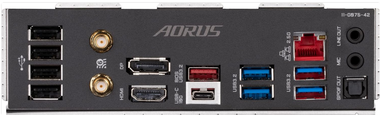
Figure 4: Rear I/O panel with various connectivity options.
