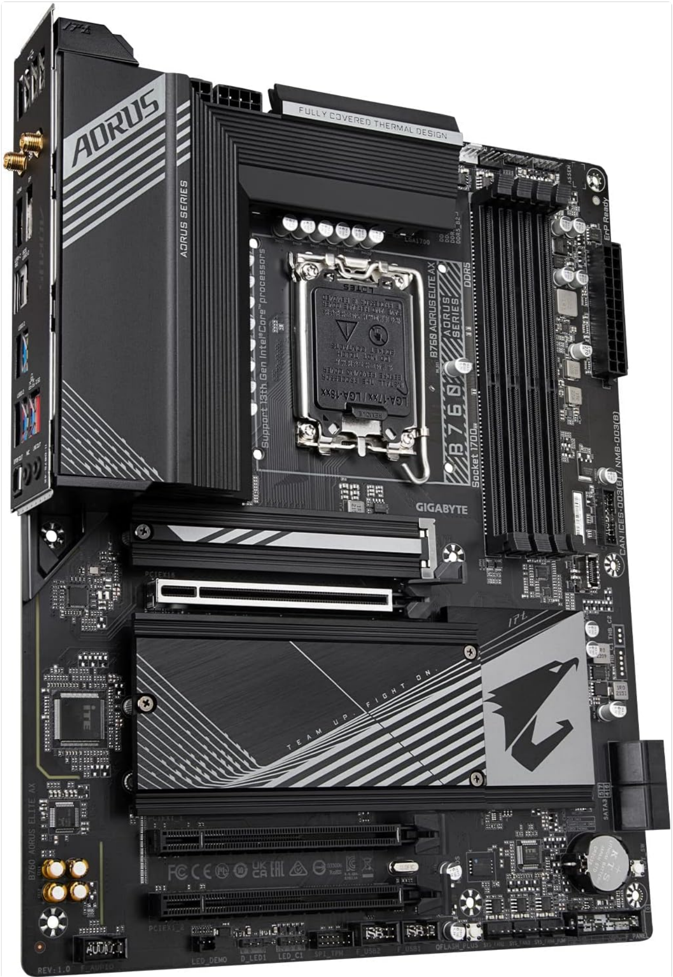
Figure 2: CPU socket (LGA 1700) and DDR5 DIMM slots on the motherboard.
