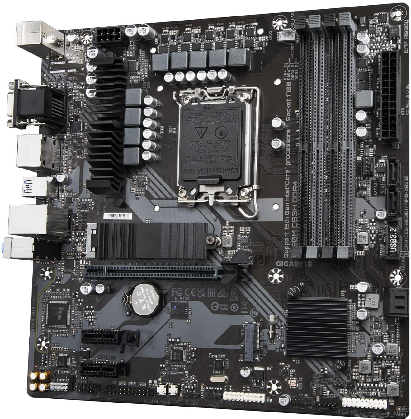
Figure 2.2: Angled view of the GIGABYTE B760M DS3H DDR4 Motherboard, showing various component slots and connectors.
