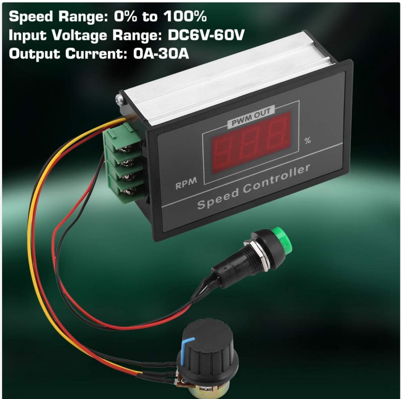
Image 3.2: The controller's digital display indicating the speed range (0% to 100%), input voltage range (DC6V-60V), and output current (0A-30A).
