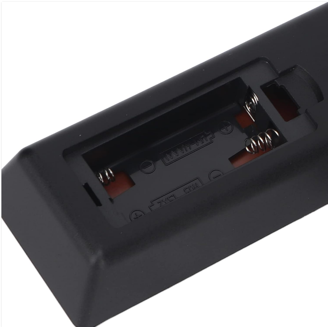
Figure 3: Close-up of the battery compartment, illustrating the correct orientation for battery insertion.
