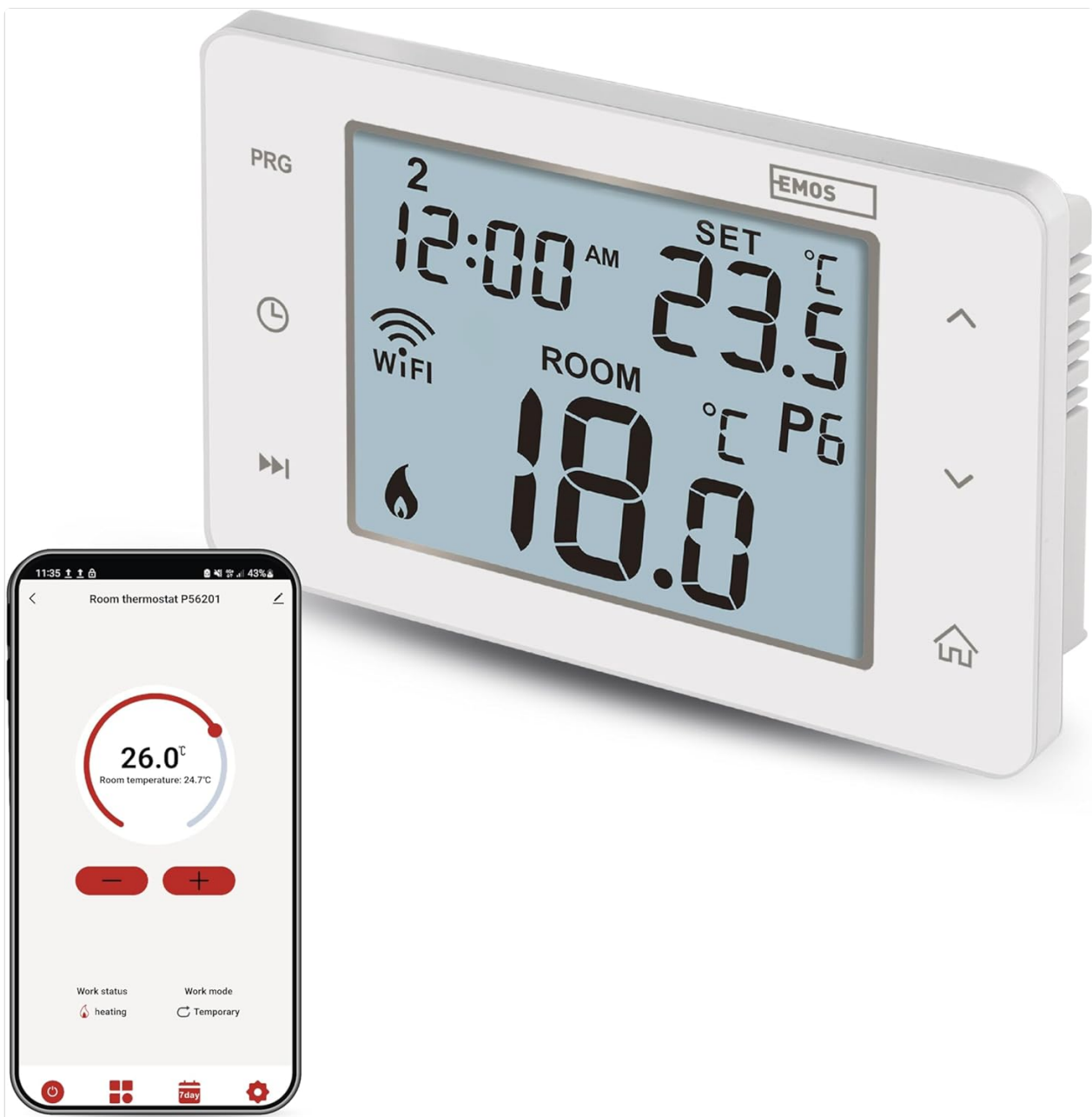
Image 1.1: EMOS GoSmart WiFi Wired Room Thermostat P56201 and its companion mobile application.
