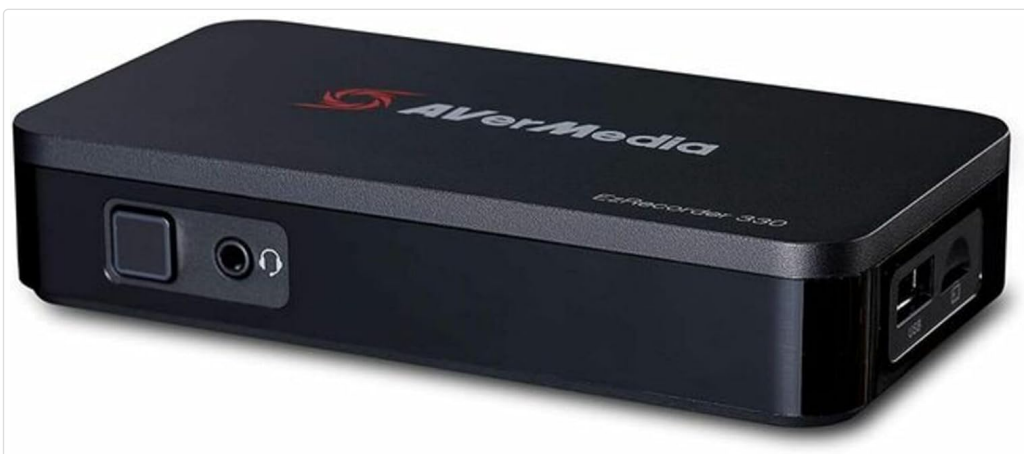
Image: The AVerMedia ER330 EzRecorder 330, a compact black rectangular device. The front panel features a square button, a 3.5mm audio input jack, and a 3.5mm headphone jack. The right side of the device shows two USB ports, one standard USB-A and one micro-USB, along with a microSD card slot.
