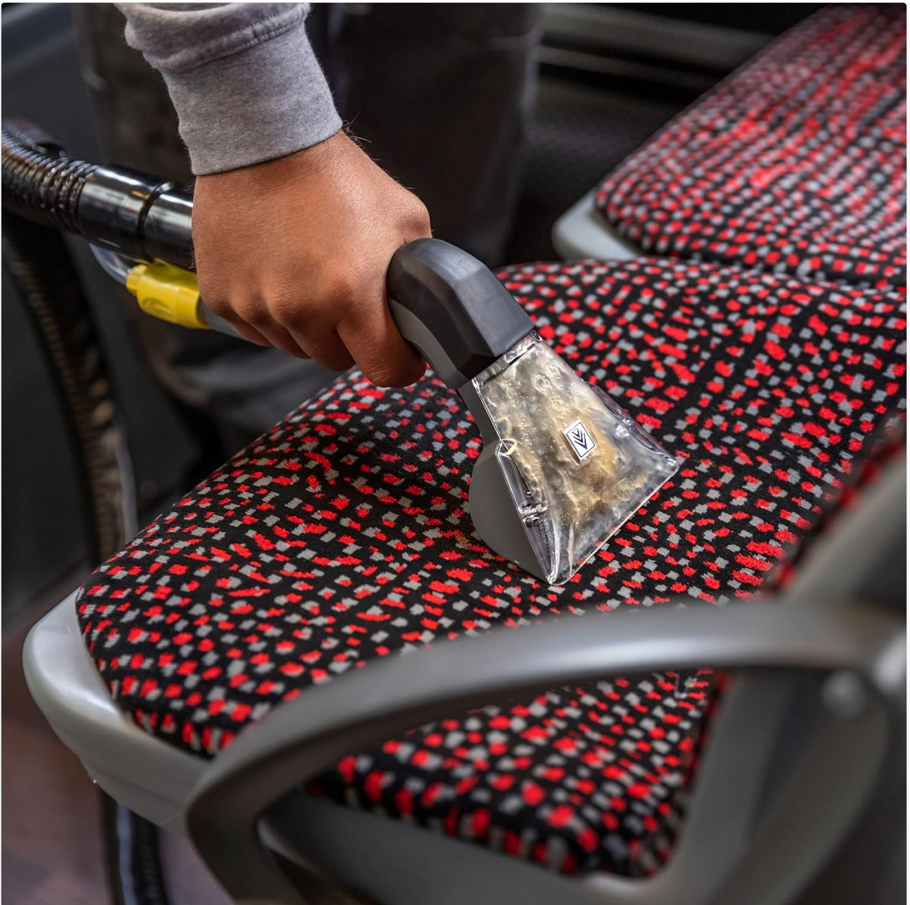
Figure 6: A close-up view of the Kärcher Puzzi 8/1 hand nozzle in action, clearly showing the extraction of dirty water from a bus seat, demonstrating the cleaning effectiveness.
