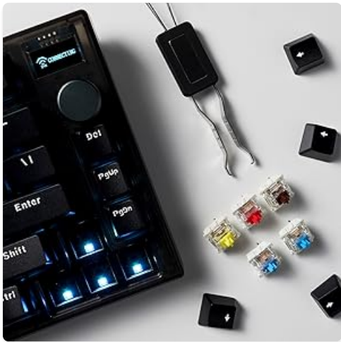
A keycap puller and various mechanical switches next to the FANTECH MAXFIT81 keyboard, illustrating the hot-swappable feature.
