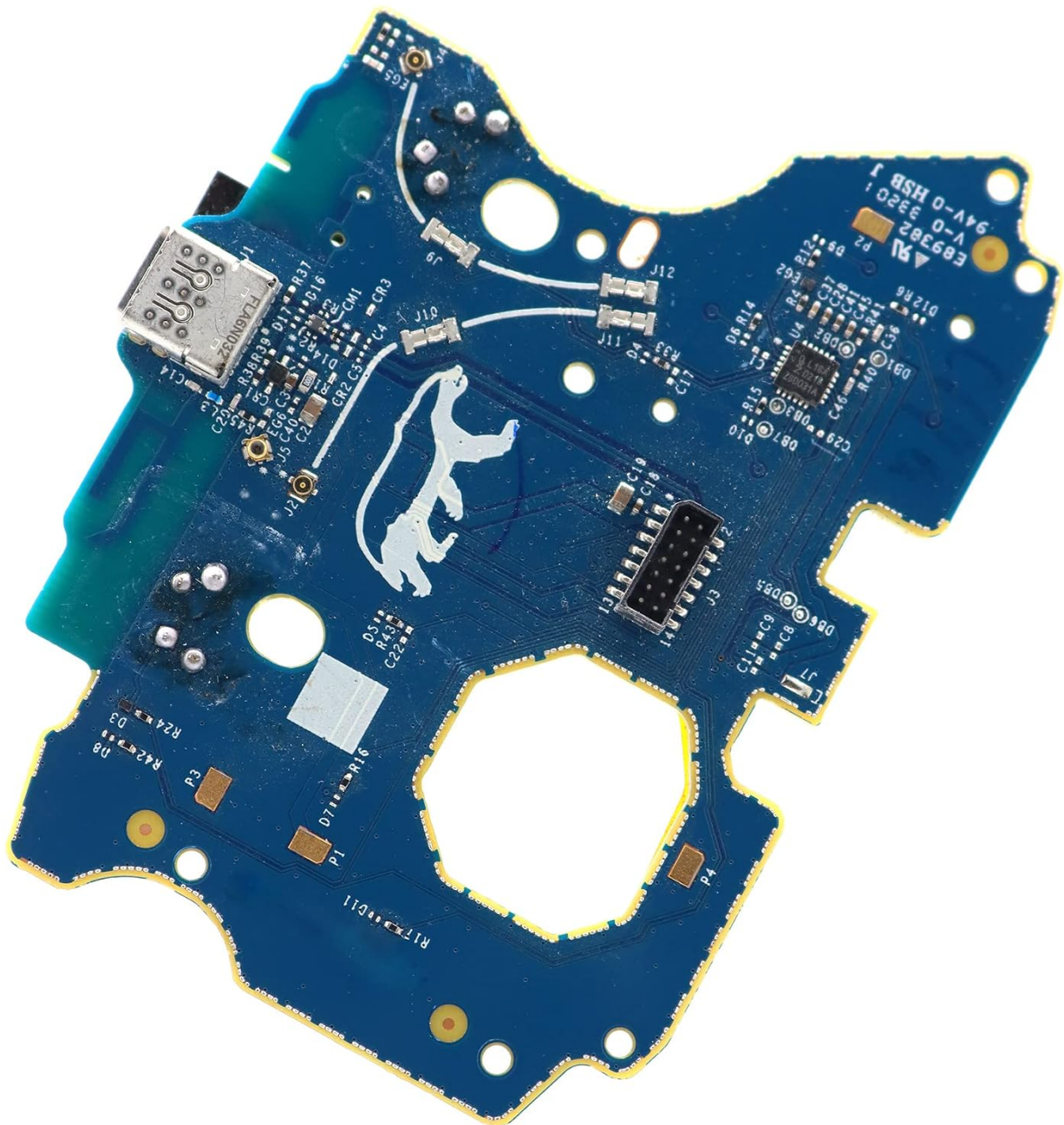
Figure 2.2: Bottom view of the M1007990 daughterboard, displaying circuit traces and connection points.
