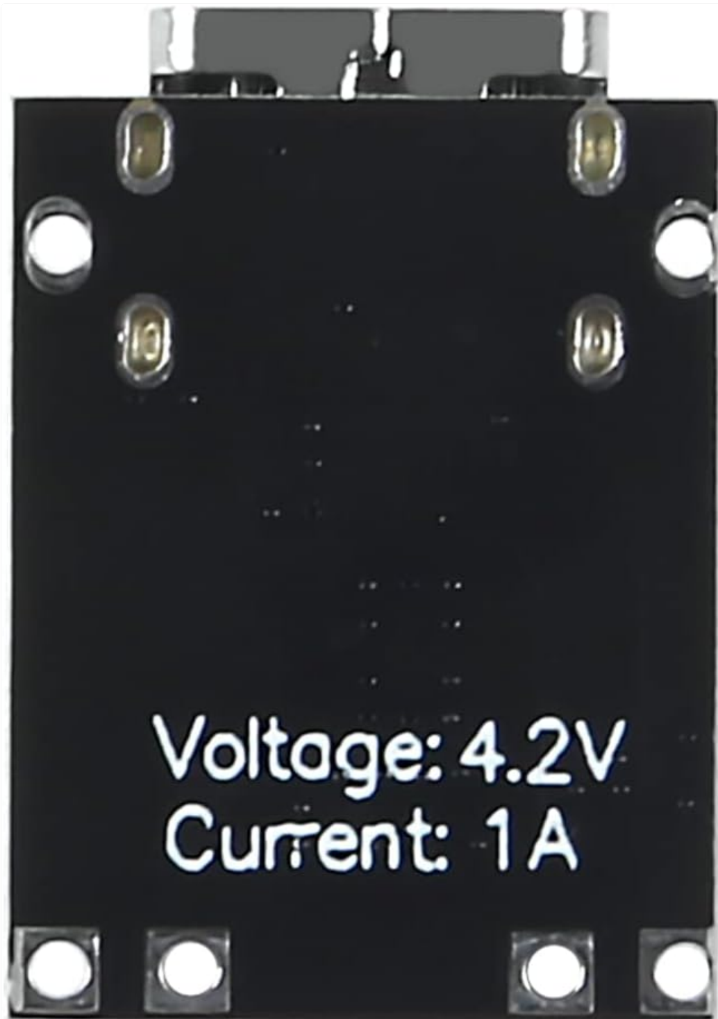
Image: Bottom view of the charger board. This view confirms the key electrical specifications printed on the board itself, specifically the 4.2V output voltage and 1A charging current.
