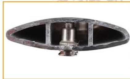
Aerodynamic structure to reduce wind noise
