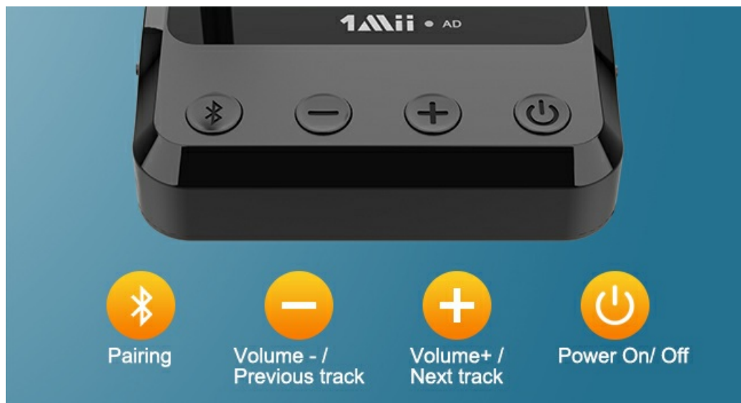
Figure 5.1: Front panel controls and LED indicators of the 1Mii B310Pro.
