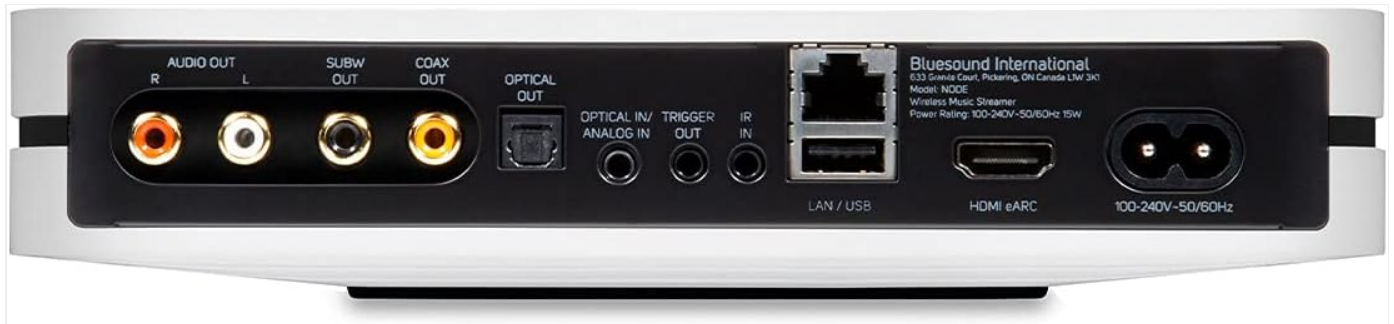
Figure 2: Rear view of the Bluesound Node (N130) displaying its comprehensive connectivity options, including Audio Out (RCA), Subwoofer Out, Coaxial Out, Optical Out, Optical In/Analog In, Trigger Out, IR In, LAN/USB, HDMI eARC, and AC power input.
