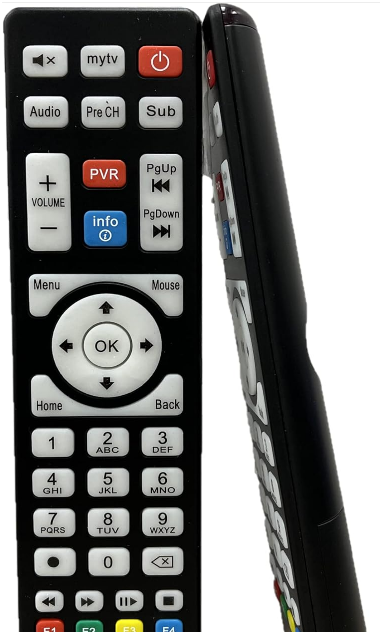
Image 2.1: Front view of the remote control, showing button layout. The battery compartment is on the reverse side.
