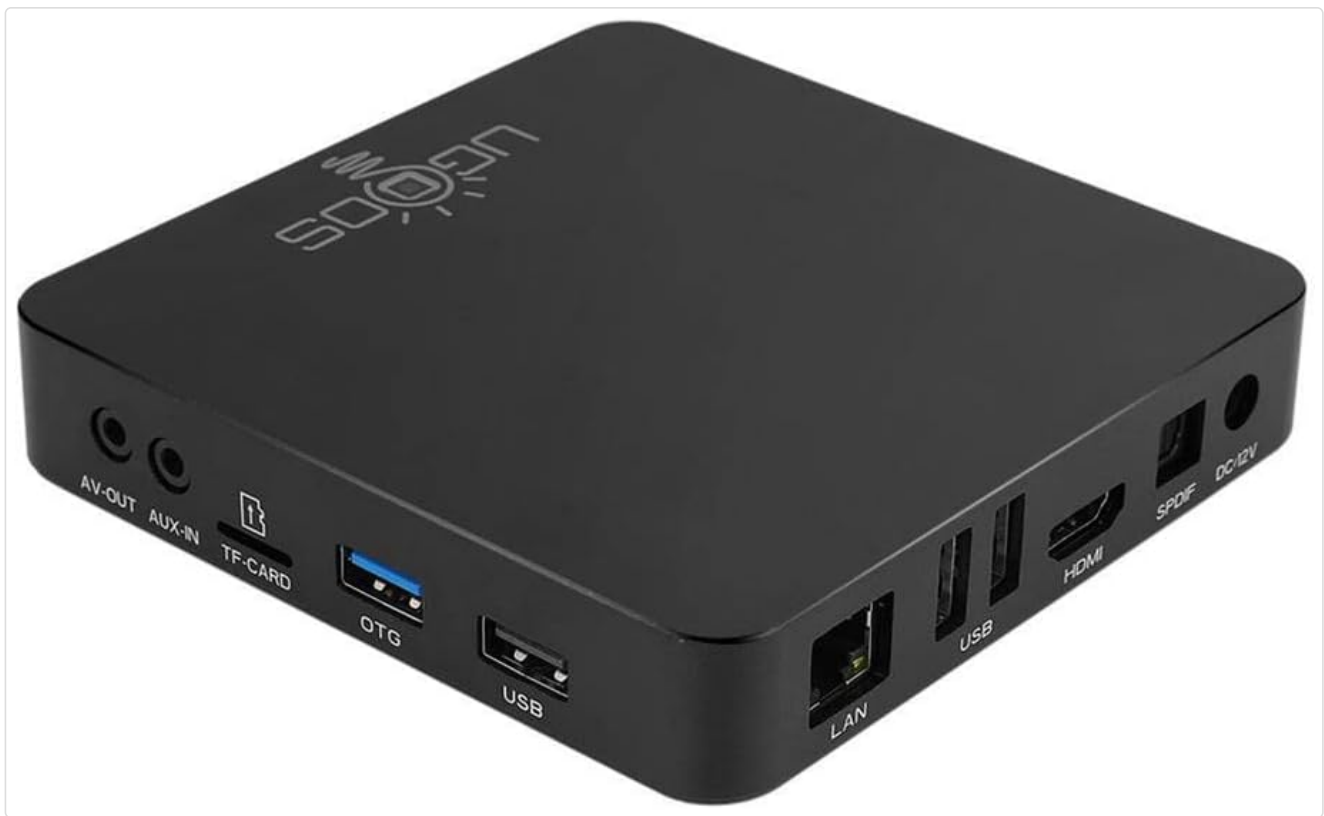
Figure 4: Rear view of the Ugoos AM6B Plus TV Box showing various connectivity ports. This image details the available ports for external connections.
