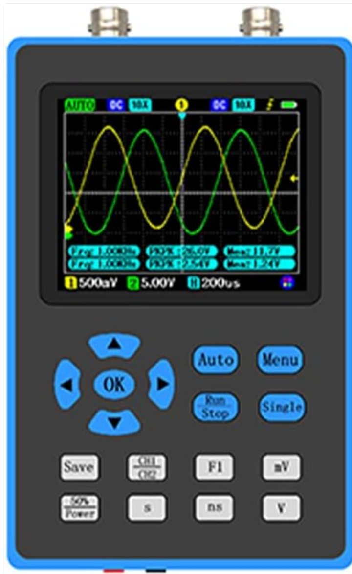
Figure 2.1: Front view of the DSO2512G Oscilloscope. The device features a central display screen showing waveform data, surrounded by control buttons for navigation, menu access, and function selection.
