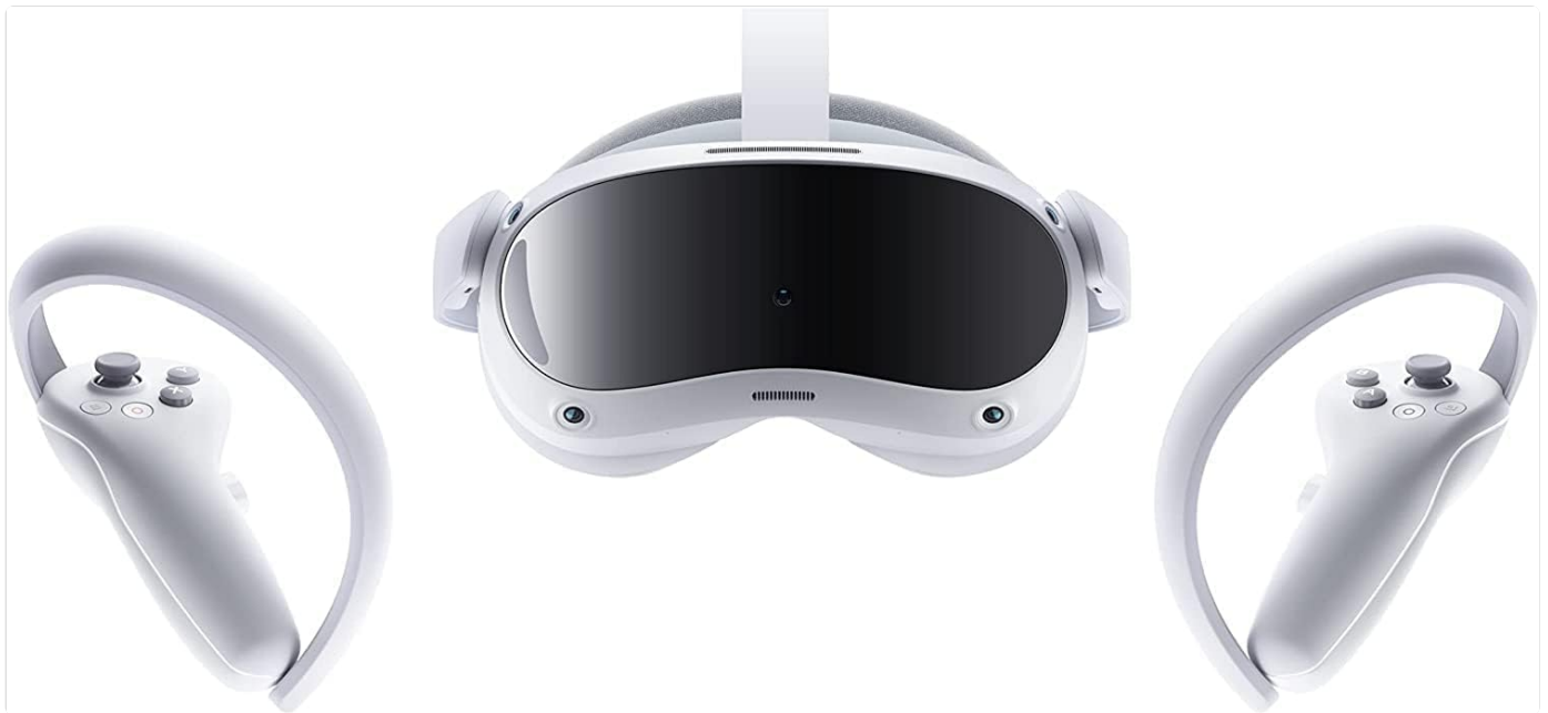
Figure 4: Front view of the Pico 4 VR Headset and its controllers, showcasing the integrated cameras for tracking.
