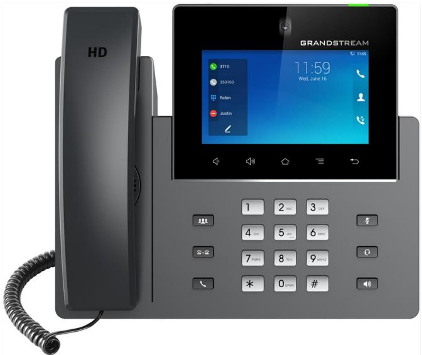
Figure 1.1: Front view of the Grandstream GXV3450 IP Video Phone, showcasing its 5-inch color touch screen, physical keypad, and handset.
