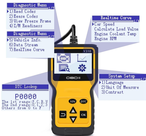
Figure 3: A composite image illustrating different screens of the V310, including the Diagnostic Menu, Realtime Curve display (Car Speed, Load Value, Coolant Temp, RPM), System Setup, and DTC Lookup with code definitions.
