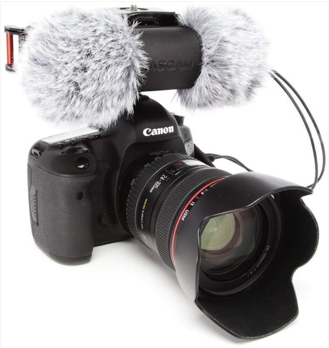
Image 5.1: The TASCAM DR-70D mounted on a DSLR camera, demonstrating a typical setup for videography.
